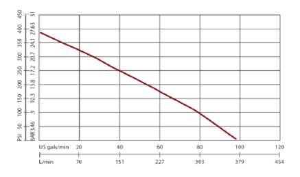
Notice how the pump curve is in the same SHAPE of the hose-lay TRIANGLE on page 8? If you keep this in the back of your mind, providing solutions to head, distance, and GPM will become MUCH easier to grasp. The higher, you go up and the farther away you get, the more pressure you need, the less flow you'll have.
