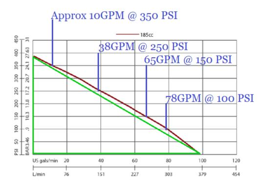
On the Bottom of the pump curve shown above, is the Gallons Per Minute from left to right, ranging from 0 to 120 GPM. On the left side is the pressure ranging from 0 psi on the bottom to 450 psi on the top. The RED Diagonal LINE is best viewed as the pump's LIMIT Line. In other words, obtaining 75 gallons per minute at 250 psi is NOT possible, nor is obtaining 10 gallons per minute at 400 psi!
